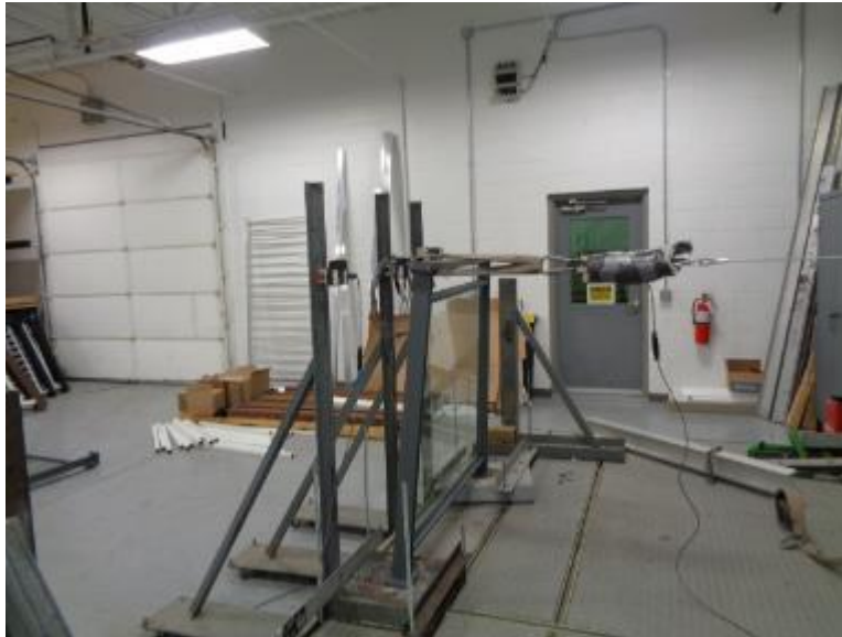
Photo No. 1 Concentrated Load Test at End of Top Rail (Bracket/Post)
