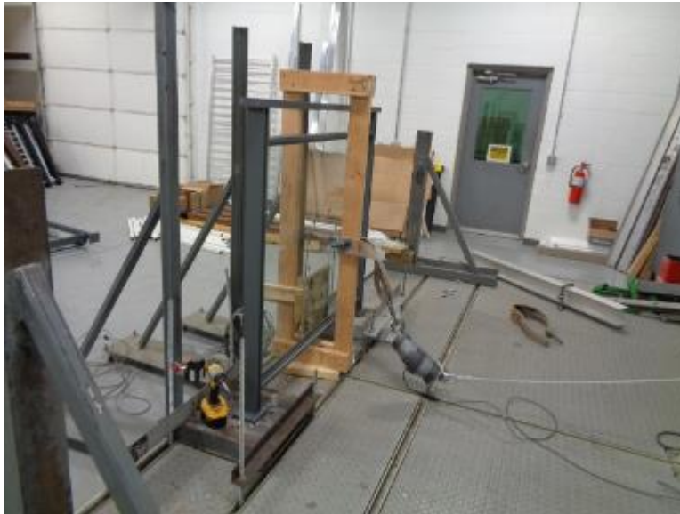
Photo No. 3 Infill Test at Bottom
