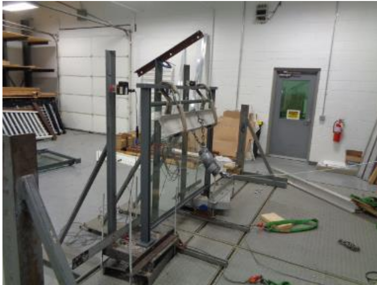
Photo No. 5 Horizontal Uniform Load Test on Top Rail
