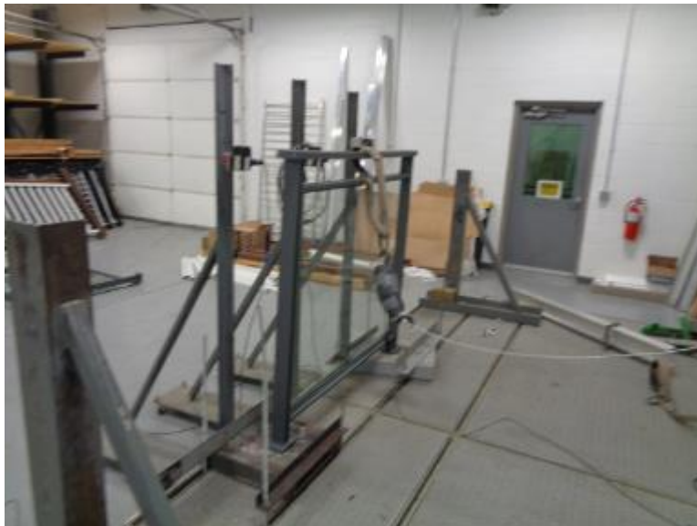
Photo No. 2 Horizontal Concentrated Load at Midspan of Top Rail
