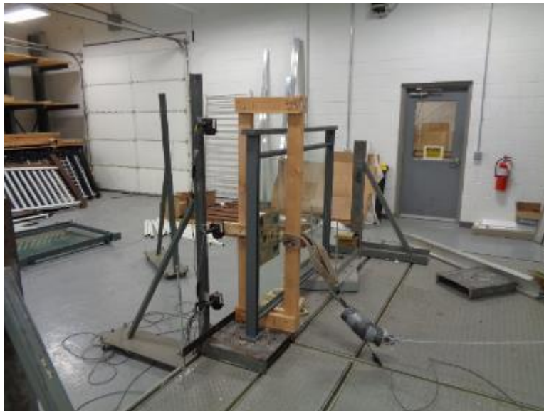
Photo No. 6 Infill Load Test at Edge
